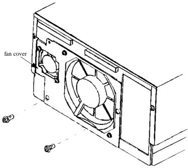
Figure 8-4. Fan Assembly
